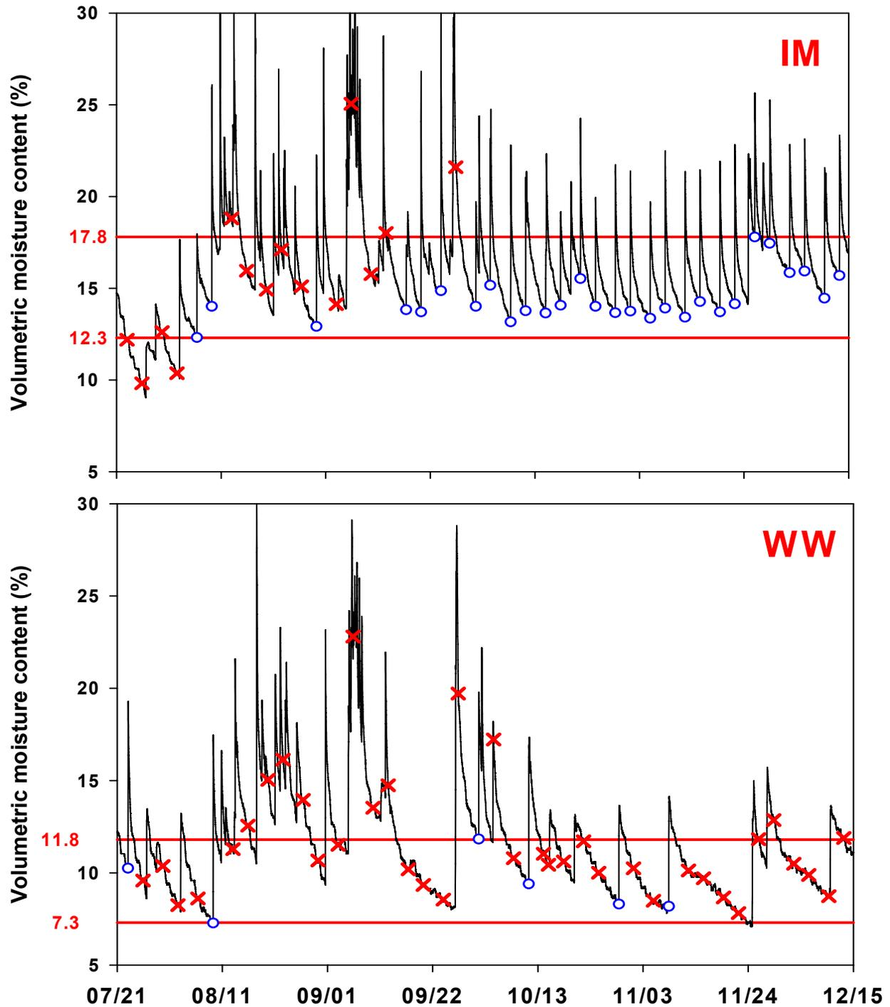
Figure 6. Volumetric moisture content ( $\theta$ ) through the experimental period of 2004, showing results of the scheduled irrigation cycles (SIC), where a red “x” represents a bypassed SIC, a blue circle represents an allowed SIC, and the red lines represent the range of  $\theta$  when the SIC were allowed; treatments Irrrometer (IM) and Water Watcher (WW). When an increment in the  $\theta$  does not have a blue circle on the bottom of the curve, it means that a rainfall event occurred.
