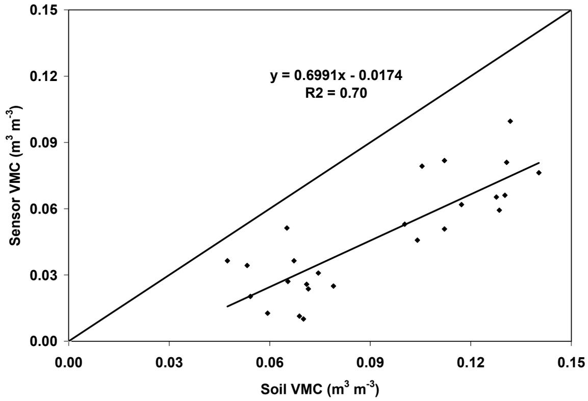
Figure 3. ECH<sub>2</sub>O calibration results for an Arredondo fine sand; linear regression (VMC= volumetric moisture content).
