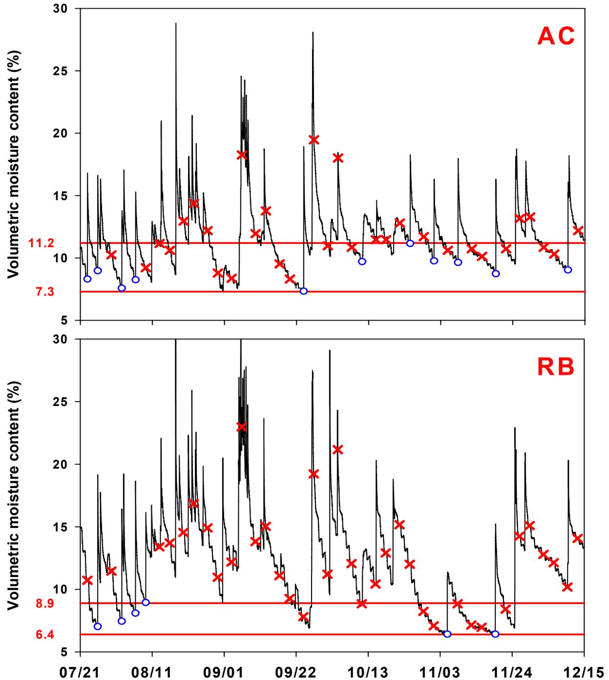
Figure 5. Volumetric moisture content ( $\theta$ ) through the experimental period of 2004, showing results of the scheduled irrigation cycles (SIC), where a red “x” represents a bypassed SIC, a blue circle represents an allowed SIC, and the red lines represent the range of  $\theta$  when the SIC were allowed; treatments Acclima (AC) and Rain Bird (RB). When an increment in the  $\theta$  does not have a blue circle on the bottom of the curve, it means that a rainfall event occurred.
